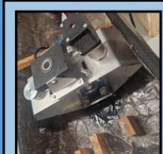
Problems arose during the installation of the system as its width barely fit the vessel. The complete system was also too high, so the lid would not close on top of the boat.
