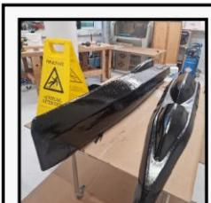
During the planning however, as can be seen in the picture to the right, the watertightness of the coating was determined to be untrustworthy. The removal of the original coat, filling and smoothening of the hull, and recoating of the vessel followed.
