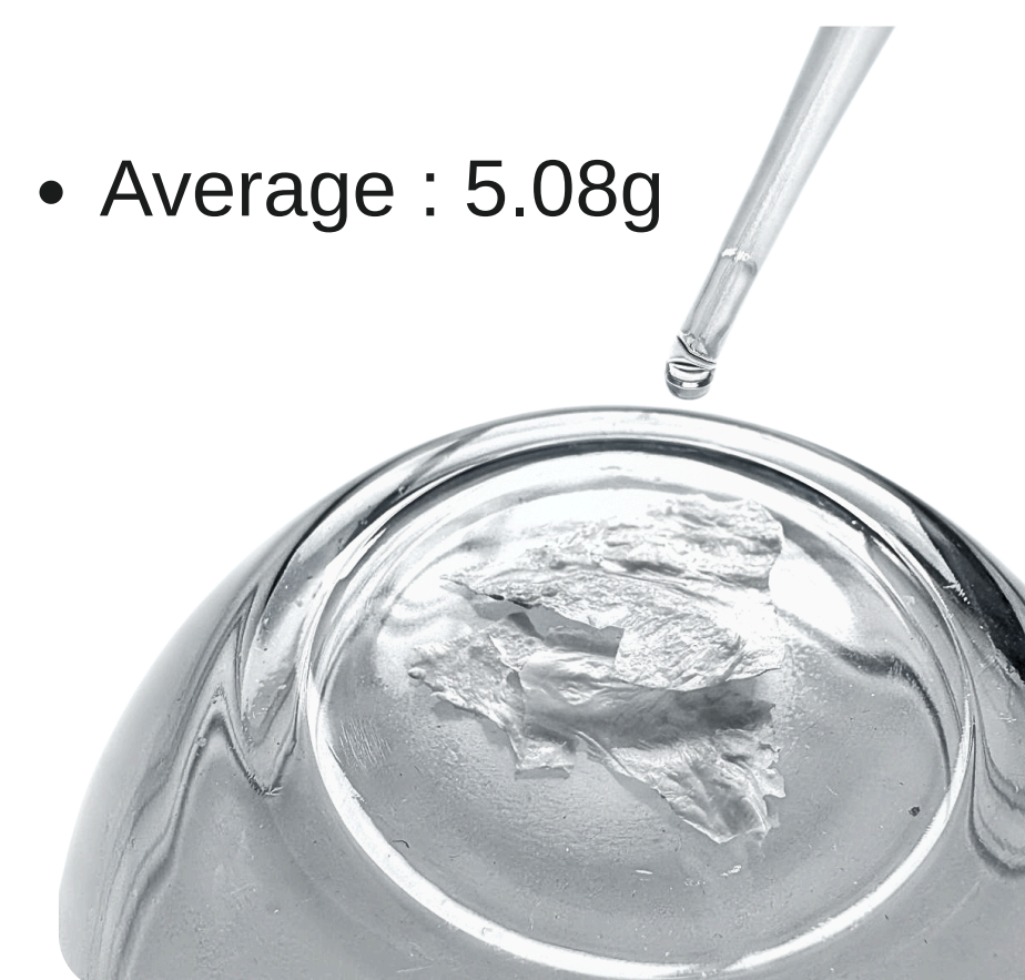
Figure 6. Dried Leachate in Contact with Acetic acid
