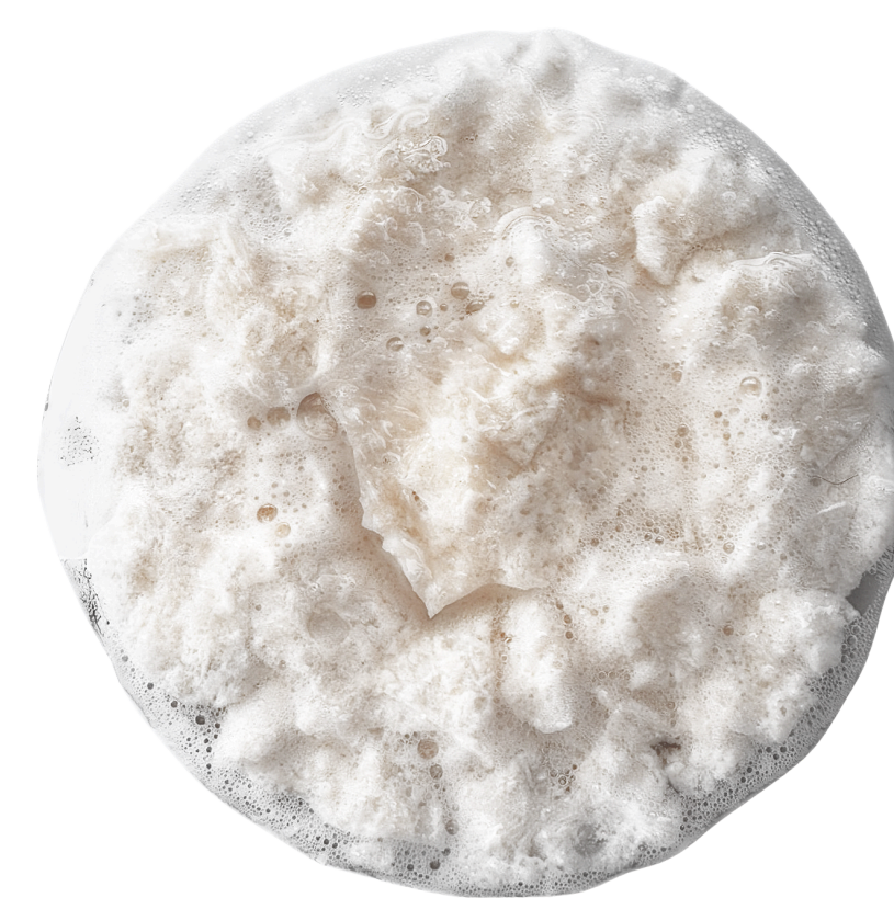
Figure 5. Efflorescence in Contact with Acetic acid indicating the presence of carbonates
